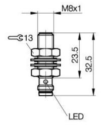
Inductive Sensors BES 516-324-E5-C-S 49 M8x1 x 32 normally-open Sn=1,5mm shielded
